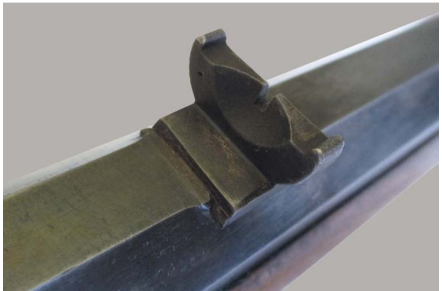
The rear sight can also be moved by tapping the base with a small brass punch.
