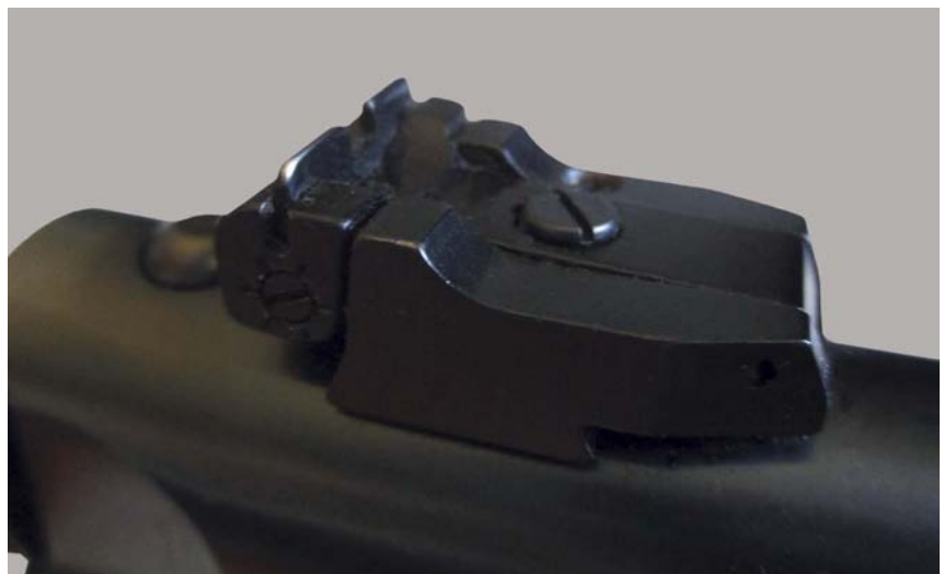
Screw adjustment for both windage and elevation is provided via the rear sight on this Ruger target pistol. The front blade is fixed because no adjustments are needed.
