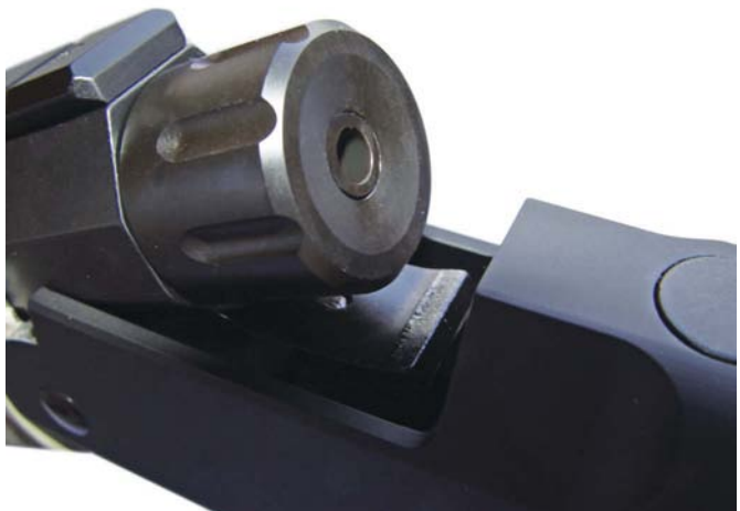
In order to prime the T/C Strike using a normal 209 shotshell primer, the action must be opened, after which the primer is placed into the hole in the retaining collar and the action is reclosed.
