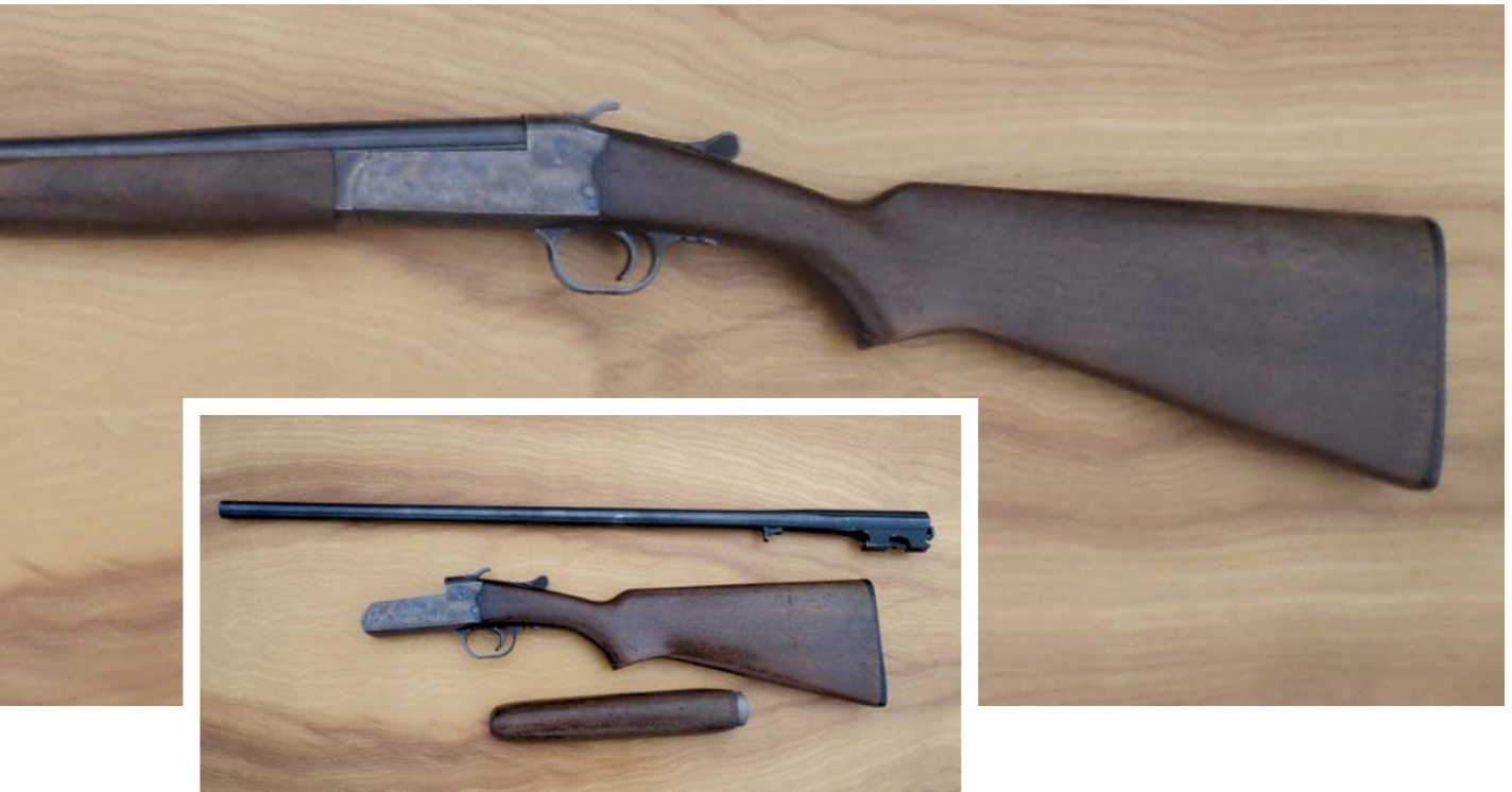
(above) A single-shot 20-gauge shotgun is disassembled into three separate pieces that can be reassembled in mere seconds.
