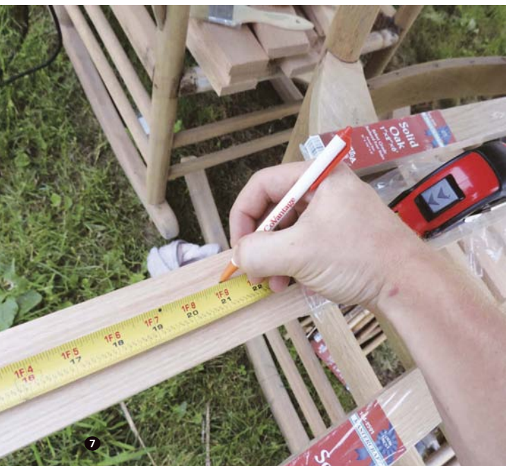
7 The oak boards are measured and marked to be cut into seat planks and backrest spindles. 8 A chop saw is used to cut the oak boards into planks and spindles. 9 The author's wife, Becca, arranges and spaces the seat planks on the chairs.
