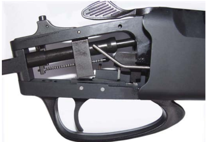
The T/C Strike’s trigger is very good quality and comes from the factory at a smidge over 4 pounds.
