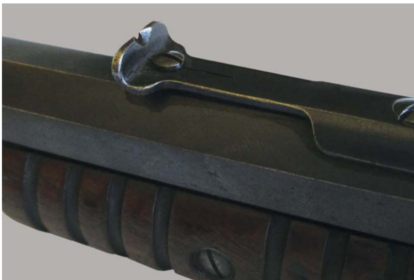
The rear sight on this old Winchester .22 rifle is equipped with a screw to adjust elevation.
